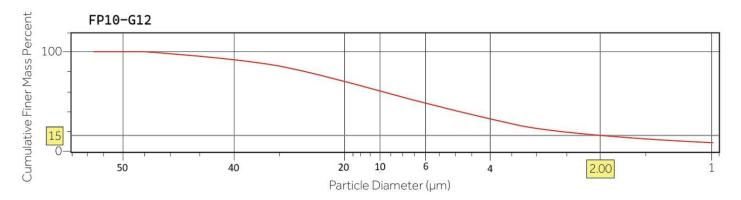
FP10 Filter aids may be applied either as precoat on the septum and/or as body feed in the liquid. As precoat, Siaba filter aid can be applied as a thin layer over the filter before the suspension is pumped to the apparatus. A precoat prevents the suspension particles from becoming so entangled in the filter medium that its resistance becomes excessive. Further, it facilitates the removal of cake at the end of the filtration cycle.
